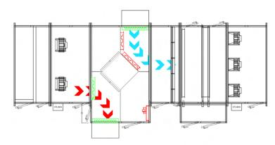
Similar operation to the wheel option, the one difference is the hood that was used for outside air intake during normal operation is now used for exhaust air during economizer operation.
