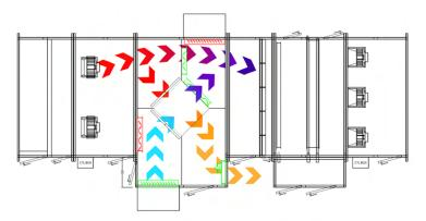
Nearly identical operation to the wheel option, the only difference being the airstreams cross each other through the enthalpy plate.
