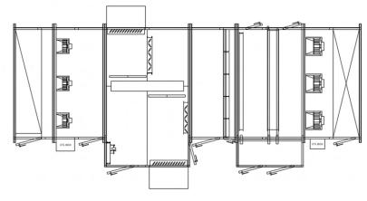
economizer and energy recovery sections into one. Utilizing a series of dampers and front loading filters, this layout is independent of return air opening location and fan type.
