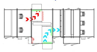
During economizer operation, the recirculation damper and exhaust louvers **close**. The return air exhausts through a hood. The outside air is drawn in, bypasses the wheel, and enters the supply tunnel.
