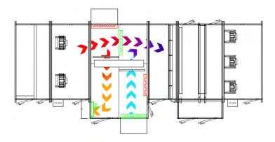
During normal operation, the return air passes through the recirculation damper and also exhausts through the energy recovery wheel. Outside air is drawn in through a hood, goes through the wheel, and mixes with the recirculation air.
